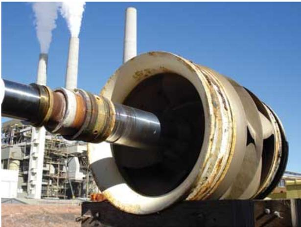
A double suction impeller for one of the cooling tower pumps. Photo, Quadna.
